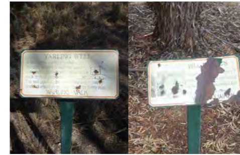
Examples of existing weathered signage including fading and coating failure.
