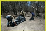
The bund contained more than 100 trees, with some trees fitted with sensors to measure tree girth, sap flow, and measure water and soil parameters. Over two weeks, 100 000 litres of fresh water was applied to the bund and a water depth of more than 30 centimetres was maintained for seven days.
