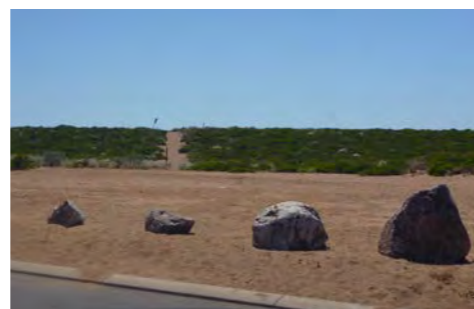
Rocks can be used as an effective and low-cost substitute for formal traffic bollards.
