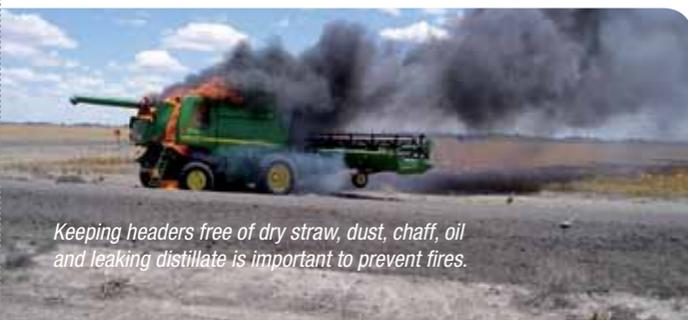
Keeping headers free of dry straw, dust, chaff, oil and leaking distillate is important to prevent fires.
