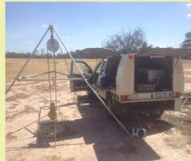
Applying the borehole nuclear magnetic resonance technique provided a unique opportunity to take a technology developed for the oil industry and apply it in environmental management to map aquifers
