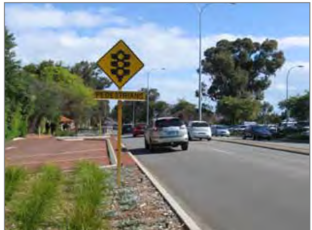
Signals Ahead (W3-3) with supplementary Crossing Ahead (W8-22) sign
