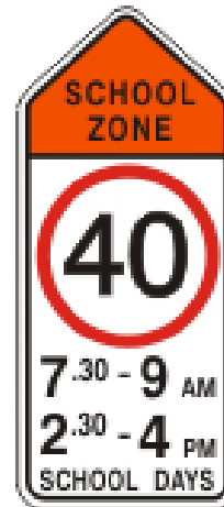
School Zone Sign placed at the start of the zone on roads fronting the school (MR-RS-15B)
