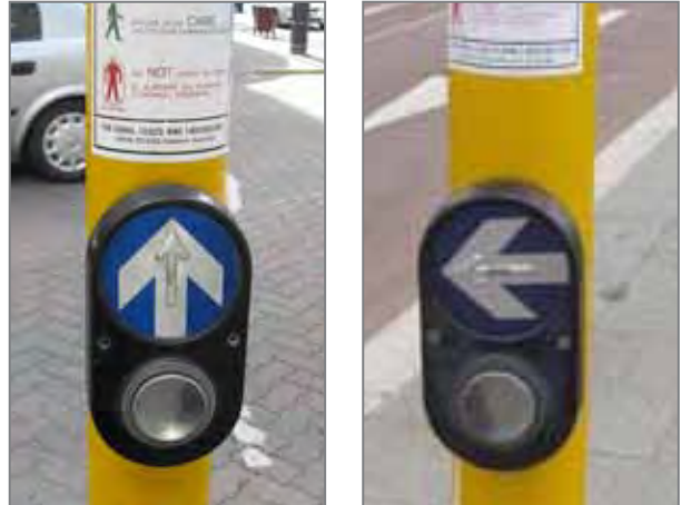
Correct push button orientation for mid-block crossings and traffic signals with an exclusive pedestrian phases
